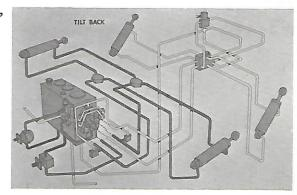
The tilt spool is moved to the right in the "tilt back" position. Oil from the pumps enters the left half of the spool, unseats the check valve, and passes to the base end of the tilt cylinders. Oil also flows into the cavity behind the regenerating check valve to keep it from opening.
