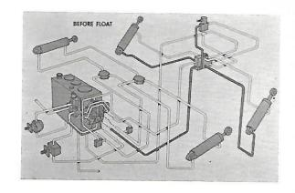
Here we see the drop valve while the bucket and arms are in the carry position. The small hole in the bottom port leads to the solenoid valve.
