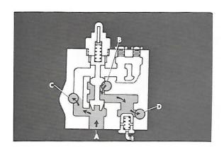
At speeds above 1500 RPM, pressure from the steering pump (A) is sufficient to displace the valve spool to a point where all of the demand oil goes to the bucket system. It is important to note that all the oil from the steering pump always goes to the steering valve.
