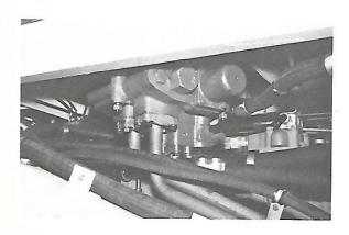
This pump supplies oil, by way of the demand valve, to the steering valve (shown) which is located almost directly below the operator's seat.
