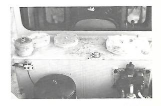
The pressure reducing valve is located on the upper left-hand corner of the tank. It reduces the air shift system pressure to 6 PSI and insures that this is the minimum pressure inside.
