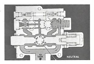
This picture shows the steering system oil flows in the neutral position.
