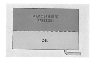
The 72-81 hydraulic tank operates on a pressurized feed and antisyphoning drain principle. In a standard tank, if a line is disconnected, all the oil would flow out of the tank due to gravity.
