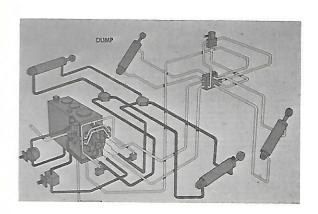
Pushing the bucket tilt control lever forward into the "dump" position allows pump oil to pass through the control valve and lines to the rod end of the tilt cylinders. The tilt cylinders retract and move the bucket forward to dump its load. Oil in the base end of the cylinders returns to the control valve. Oil returns to tank or to the rod end of the cylinders, if pumps cannot supply oil fast enough.
