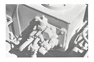
This is a cutaway view of the demand valve showing the inlet and outlet ports. P-1 is the steering pump and P-2 is the demand pump. The outlet port labeled P-1 and P-2 goes to the steering valve and the outlet port labeled P-2 goes to the bucket hydraulic valve.
