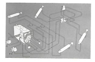
A hydraulic tank, two hydraulic pumps, a control valve, a demand valve, two lift cylinders, two tilt cylinders, a drop valve, a solenoid valve, and two relief valves.
