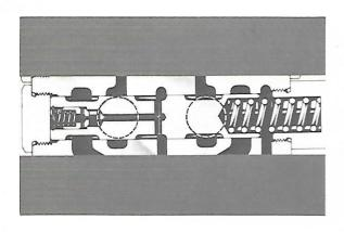
The plunger directs oil to the appropriate ends of the steering cylinders. It consists of the plunger itself, a return spring, a poppet, a poppet spring, a snap ring, and a washer.
