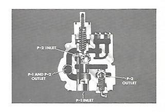
This is how the demand valve operates. At an engine speed of less than 1000 RPM the steering pump pressure is not great enough to move the spool inside the valve significantly. Under these circumstances, the spool directs all of the oil from both pumps (A & B) to the steering valve (C).
