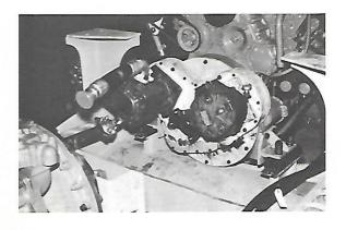
Two gear-type pumps are driven by the power take-off (PTO) unit located on the rear of the engine. The larger pump on the left is the main hydraulic pump and the one on the right is the demand pump.
