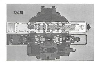
This cutaway shows the lift spool pulled into the "raise" position. When the spool is moved to the right, pump oil passes through the central passage of the valve and enters the spool through the ports at the left. The check valve that holds the pressure in the base end is unseated and oil is sent through it to raise the lift arms. Displaced oil from the rod end enters the valve at the port at the upper right, enters the spool and returns to the tank.
