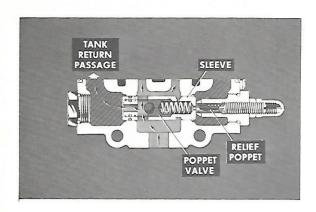
This allows the poppet valve to shift towards the right and draw the ball off its seat. Oil flows out the tank return passage to the extent necessary to receive the high pressure problem.
