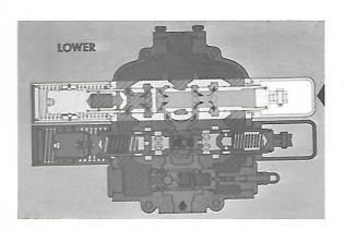
When the lift spool is moved to the left into the "lower" position, pump oil passes through the central passage and enters the ports in the lift spool. The oil then passes through the spool and to the ports leading to the rod end of the lift cylinders. Oil returning from the base ends enters the valve and valve spool at the left, unseats a check valve, and flows from the spool into the return-to-tank passage.
