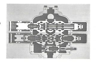
The lower valve spool controls the bucket dumping and rolling back. It has one detent (tilt back) and is self-centering when out of detent. The spool has a check valve in each end to hold pressure in either end when shifting the tilt lever from the "hold" position. The left port goes to the base end of the tilt cylinder and the right port to the rod end. This spool is a regenerative type, which means that the spool uses oil from one end of the cylinder to help the pump fill the other end.
