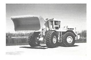
And the tilt cylinders which are located on the outboard side of the lift arms.
