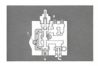
As engine speed varies between 1000 and 1500 RPM, so does the position of the valve spool. At 1000 RPM the spool begins to allow some of the oil from the demand pump (B) to flow into the bucket hydraulic control valve (D). As speed continues to increase, so does the percentage of the demand pump's output which goes into the bucket system. When the engine approaches 1500 RPM, almost all of the demand pump's oil is allocated to the hydraulic control valve.
