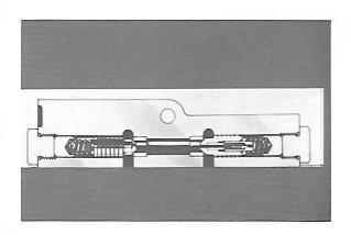
The purpose of the two double relief valves is to relieve shock loads in excess of 2400 PSI placed on the steering cylinders. Each of these valve assemblies consists of a seat, the valve itself, a spring, a plug, an "O" ring, and an end cap.
