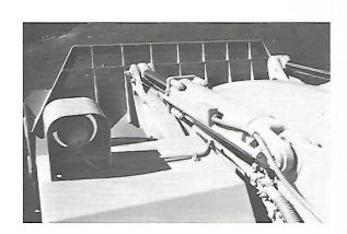
The demand pump supplies the demand valve (shown) on the front of the hydraulic tank, which assigns the fluid from the pump to the bucket hydraulic system and the steering system. The portion which each system receives depends on engine RPM.
