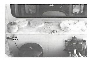
The 62-1/2 gallon hydraulic tank is located immediately behind the operator's compartment.
