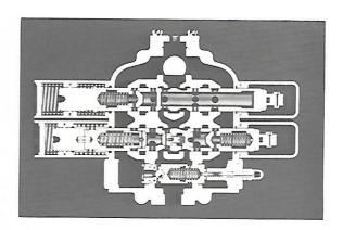
The hydraulic control valve is a two-spool type with a 2500 PSI relief valve. The upper spool controls the raise, hold, lower, and float positions on the bucket arms while the lower spool controls the rollback, hold, and dump positions of the bucket.
