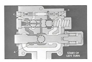
when making a left turn, the control spool is moved into the valve housing shutting off the right side passages to the pressurized oil. The oil flows up the left side and is blocked by the plunger.
