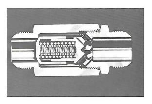
The one-way check valve is found on the bottom of the hydraulic tank between the two T fittings. It protects the oil cooler from high pressure by by-passing it. The poppet begins to crack at 45 PSI and is fully open at 65 PSI.
