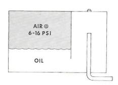
In a pressurized feed and anti-syphoning drain type tank, the air pressure from the pressure reducing valve forces the oil level down in one half of the tank (in this case the left) and, as a result, up in the other half. The oil then flows down the high-rise tube and to the pumps, all under pressure.
