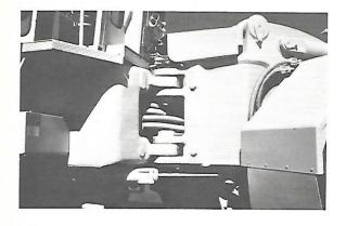
The steering valve controls the steering cylinders shown underneath the pivot area.
