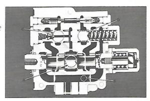
The purpose of the control spool is to direct oil to the plunger. The apparatus on the right hand side is a self-centering device containing a spring, two end washers, and a sleeve which limits the travel of the spool.
