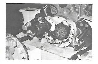
Again, as was in the steering system discussion, we have already discussed many of these components. As a small review, the main hydraulic pump is located on the left half of the engine mounted PTO, the demand pump is located on the right.
