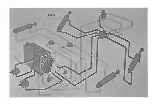
When the bucket arm control lever is pulled back to the "raise" position, oil flow from the pumps passes through the control valves and lines to the drop valve. From the drop valve, the oil goes to the base end of the lift cylinders to extend them. This raises the lift arms since they are pinned to the rod end. Oil from the rod end is sent through the drop valve, and the control valve back to the tank.
