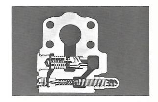
Pressurized oil which has passed through the relief valve enters the main steering valve at Port A. In a neutral position, the valve control spool is centered and oil flows around the control spool and into the outlet passage which is connected to the oil cooler.
