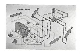
When the solenoid valve is shifted, pilot pressure from the bottom port of the drop valve is allowed to flow through the solenoid valve and back to the left end of the drop valve where it shifts the piston, rod, and bottom poppet. This allows bucket carry oil in the base end of the lift cylinders to shift the upper poppet and pass into the upper port of the drop valve into the rod end of the lift cylinder to fill the void as the bucket drops.
