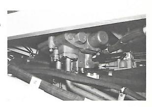
The steering valve consists of a control spool (at the bottom), a plunger (in the middle), and two double relief valve assemblies. Port A is the high pressure inlet from the main system relief valve (which is shadowed in white). Port B is the return to tank port for that relief valve. It empties into the passage that returns steering oil to tank through the port at the bottom of the picture. Ports C and D are connected to the steering cylinders.
