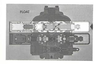
When the lift spool is pushed into float position, the valve passages leading to both ends of the lift cylinders are open to each other, to pump pressure, and to the return-to-tank passage.
