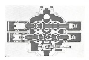
When the pressure of the oil inside the sleeve (which is the same as system pressure) exceeds 2500 PSI, the relief poppet is unseated and it allows some of the oil to return to tank. As in other pilot relief valves we have studied, a low pressure situation is now created.
