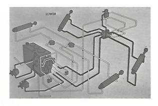
When the bucket arm control lever is pushed forward to the "lower" position, oil from the pumps passes through the control valve and lines to the drop valve. From the drop valve, oil goes to the rod end of the lift cylinders and retracts them. This lowers the lift arms. Oil from the base end of the cylinders is sent through the drop valve to the control valve and back to the tank.
