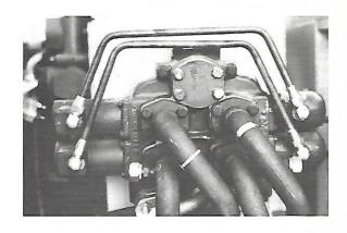
It controls the lift cylinders shown at the front of this unit
