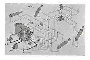
Here we can see how the valve spool blocks the passages leading to the lift and tilt cylinders.
