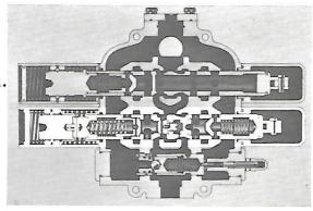
The pilot operated relief valve which controls the bucket hydraulic system pressure is located in the bottom part of the control valve housing.
