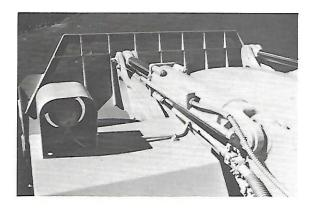
The last group of items common to both systems are the hydraulic cylinders. This tilt cylinder is a common example. The base end is usually attached to a fixed frame, whereas the rod end is secured to that which is to be moved.
