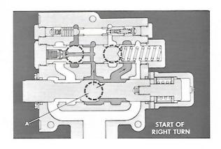
In a right turn, the steering valve control spool is slowly pulled out of the steering valve housing up to a maximum of .31 inches. This movement closes off the left side of the main oil passage. Oil enters the housing at Port A, flows into the right hand passage and is dead-ended at the plunger.
