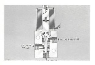
The solenoid valve, when in its normal position, has its inner spool aligned so that the pilot pressure (a small amount of oil tapped from the plumbing of the base end of the lift cylinders), is deadended. However, when the valve is shifted, pilot pressure is directed to the drop valve.
