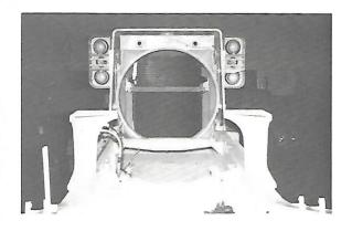
The steering system oil cooler is the larger of the two radiator type coolers located in front of the engine radiator. Remember that only steering oil passes through this cooler.
